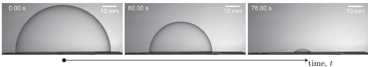
Figure 1: The photographs illustrate one of the three scenarios of shrinking surface bubbles: in this case, a bubble remains hemispherical when it shrinks.
